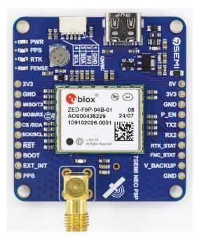
The **7Semi ZED-F9P Dual-band GNSS RTK SMA Modem Board** is a high-precision GNSS solution designed to deliver centimeter-level positioning accuracy. Built around the **u-blox ZED-F9P** module, this modem board offers seamless integration with multi-GNSS constellations and real-time kinematic (RTK) capabilities. Its versatile interfaces and compact design make it ideal for industrial, UAV, and IoT applications.
