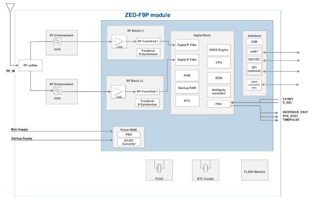
The block diagram below illustrates the integration of the **u-blox ZED-F9P module** and the board's external interfaces:
