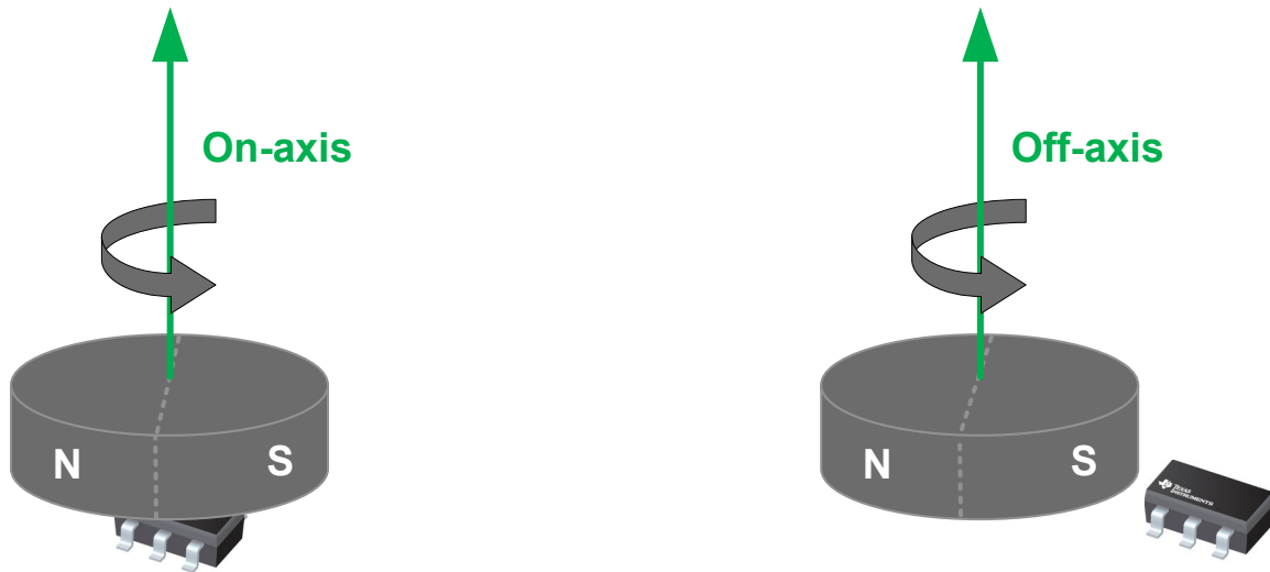
Figure 7-16. On-Axis vs. Off-Axis Angle Measurements
