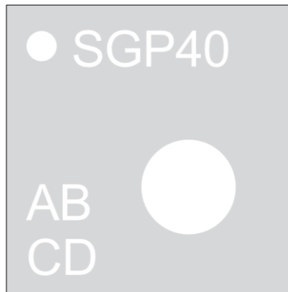
Figure 11 Top view of the SGP40 illustrating the laser marking.
